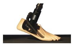
The eliteVT smoothly manages the requirements of walking and running by combining the properties of the axial spring and the foot springs. The result is a biomimetic balance similar to that provided by the combined tibial muscle and foot arch action in the natural foot.
