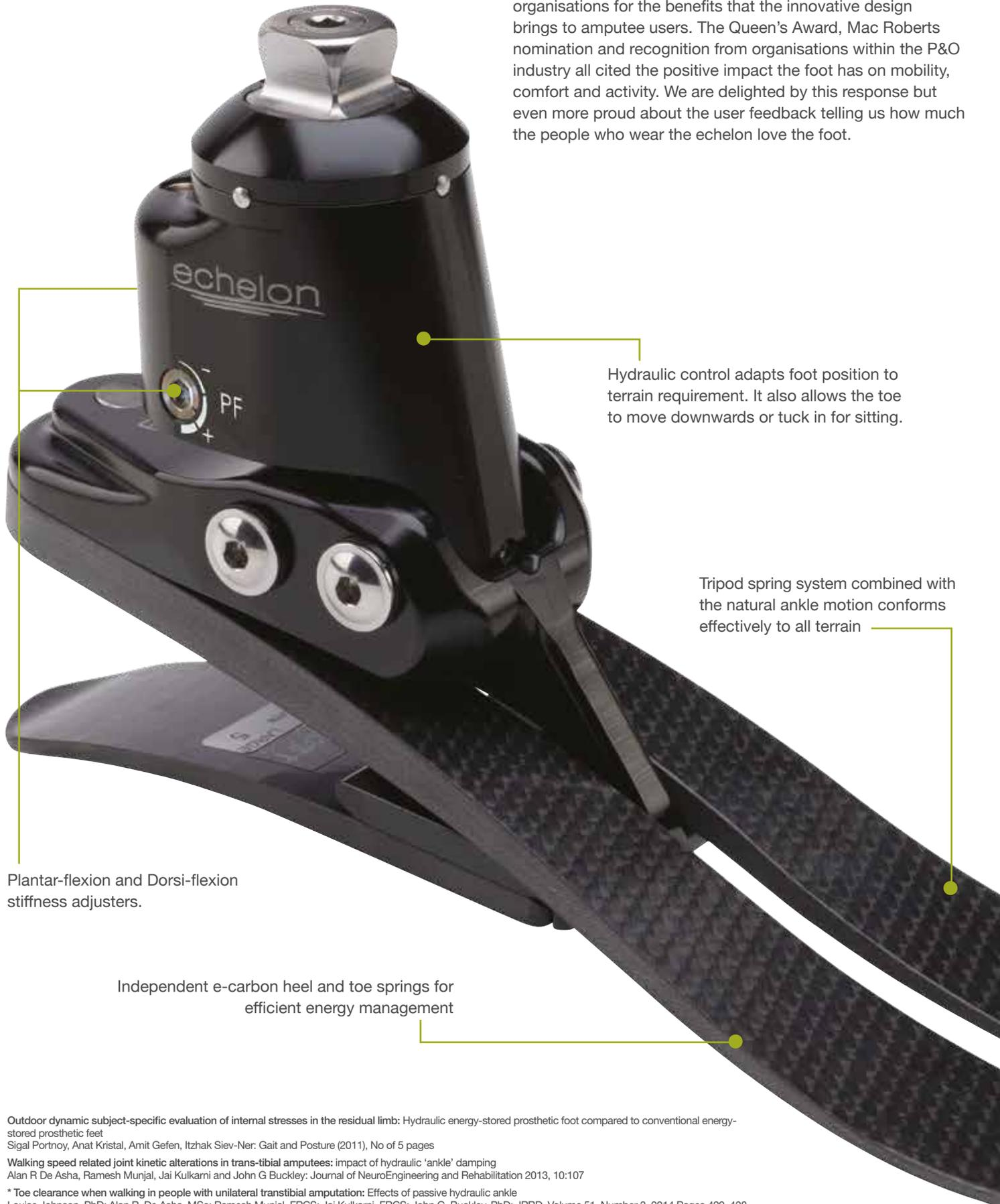
Hydraulic control adapts foot position to terrain requirement. It also allows the toe to move downwards or tuck in for sitting.
